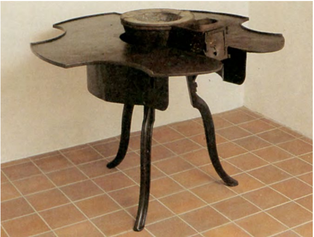
Fig. 19 Worktable for typecasting. From the Berling collection, Kulturen.
